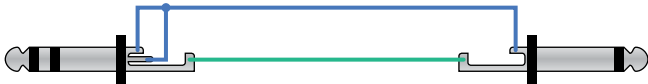
Figure 10: Tip and ring of the TRS connector will need to be connected here.
